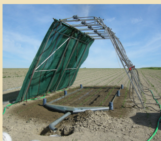
Regensimulator BAW Petzenkirchen (Variante CT) BWSB/WALLNER
